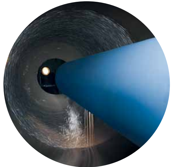
Centrifugal casting process patented by HOBAS
